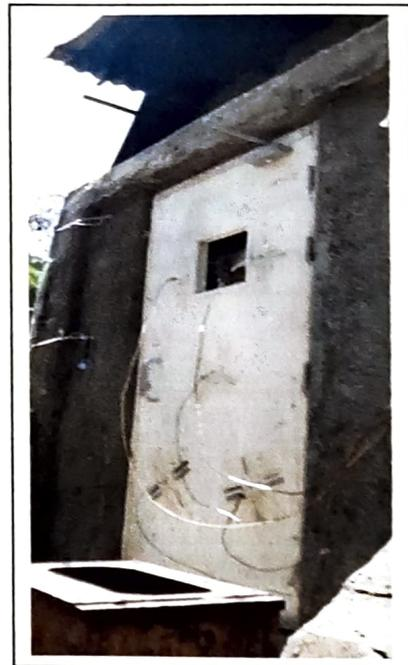
Photograph 2: Photograph of the thermocouples mounted on the Door
