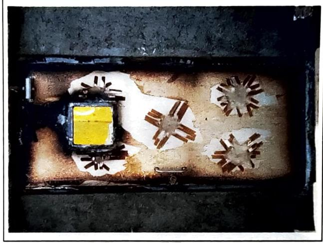
Photograph 4: Photograph of Un-exposed Side of Door
